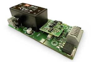
The **DALI TW8** is a DALI compatible device (device type 8), especially designed to allow for the Tunable-White control of LED modules through a DALI interface. For correct function an external LED driver is required.
